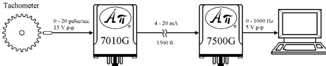
The tachometer output (24 pulse/rev x 50 rev/min x 1 min/60 sec = 20 pulse/sec) is converted to a 4-20 mADC signal by the **API 7010 G** Isolated Frequency to DC Transmitter module. At the computer, the 4-20 mADC signal is converted by the **API 7500 G** Field Selectable Isolated DC to Frequency Transmitter module to a frequency of 0-1000 Hz.
