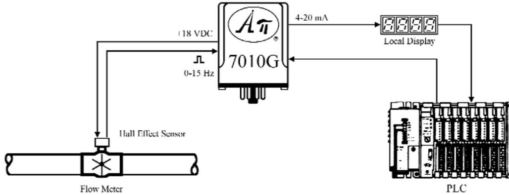
An **API 7010 G** Isolated Frequency to DC Transmitter module provides the DC power for the Hall Effect sensor from its built-in loop excitation supply and converts the 0-15 Hz flow signal into a 4-20 mA signal to drive the local display and the PLC. The 2000 VRMS isolation protects against unwanted ground loops and electrical noise.
