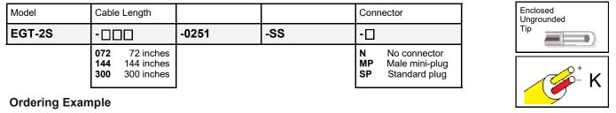
EGT-2S-072-0251-SS-N: 72 inch long cable, Type K thermocouple, no connector
