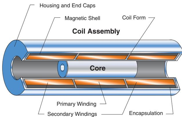
The moving element of an LVDT is a separate tubular armature of magnetically permeable material called the core. The core is free to move axially within the coil's bore, and is mechanically coupled to the object whose position is being measured. The bore is large enough to provide radial clearance between the core and coil with no physical contact.
