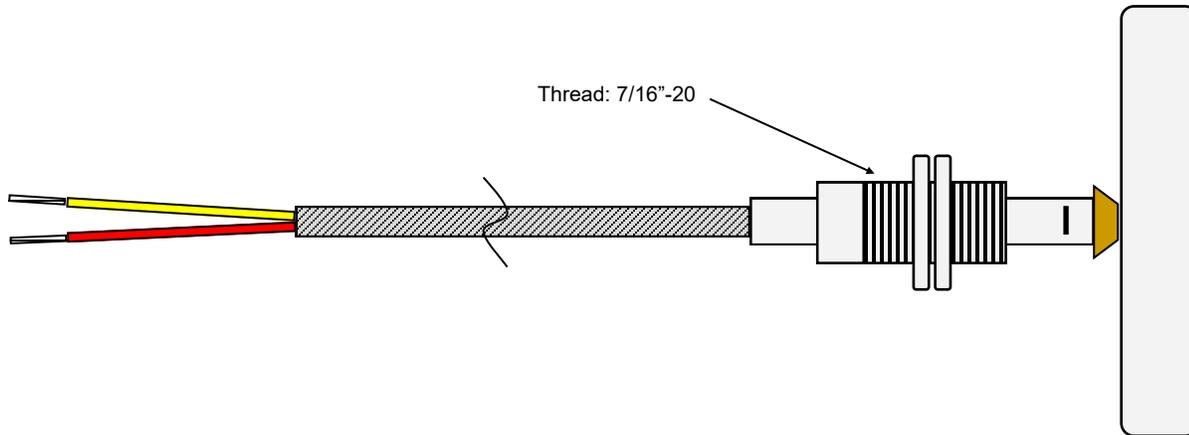
1. Install sensor so tip is lightly touching rotor surface
